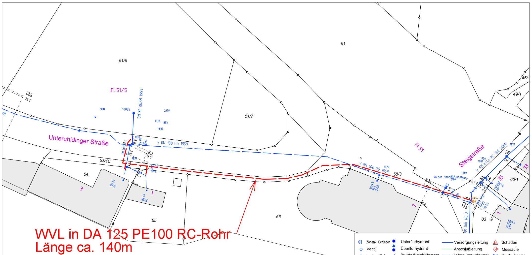
**WVL in DA 125 PE100 RC-Rohr
